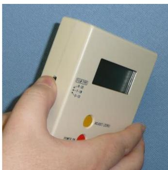
\* If the selected type of the leaf selection slide switch does not match the actual type of OptoLeaf to be measured, correct measurement cannot be performed.
