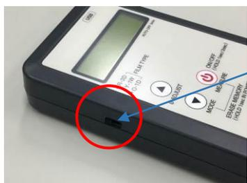
\* If the selected type of the leaf selection slide switch does not match the actual type of OptoLeaf to be measured, correct measurement cannot be obtained.
