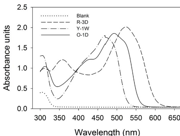
Fig. 1: Absorbance spectra of the three light sensitive film types, and blank tricellulose acetate substrate.
